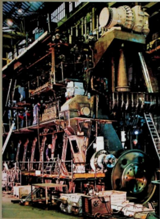
A two-stroke diesel engine type ACEC-M.A.N. K65290/160A at test bed (19 200 H.P. - 122 rpm). This engine is sold to the shipyard Bocchetti for installation in the bulk carrier "EEKLD".
