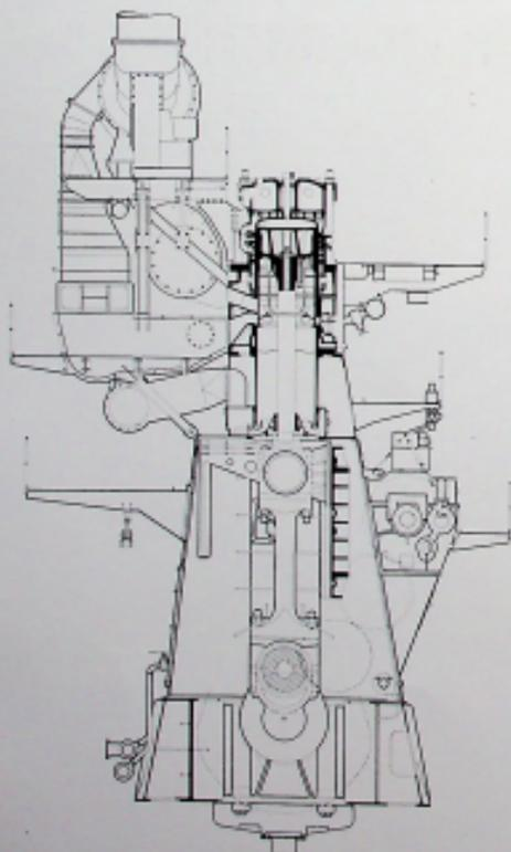
Cross-section of a two-stroke diesel engine type ACEC-M.A.N. K10 SZ 105/180 (40 000 H.P. - 107 rpm).
