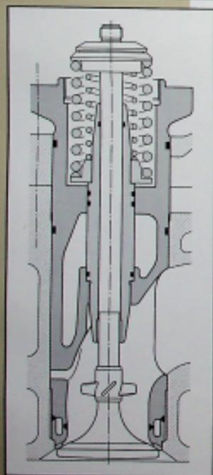
Exhaust valve of a V52/55A four-stroke engine.
