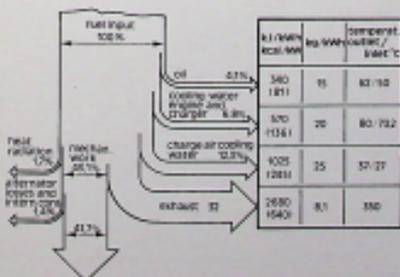
Diesel power plant with heat recovery system for heating services.
