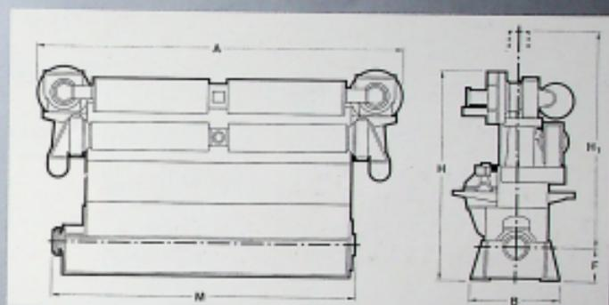
**KSZ 70/125** — 1520 kW/cyl. — 145 rpm —  $C_m = 6.04$  m/s —  $p_e = 13.1$  bar.
