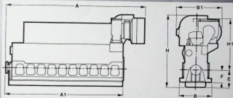
**L-V 32/36 — 370 kW/cyl. — 750 rpm —  $C_m = 9.0$  m/s —  $p_e = 20.4$  bar.**
