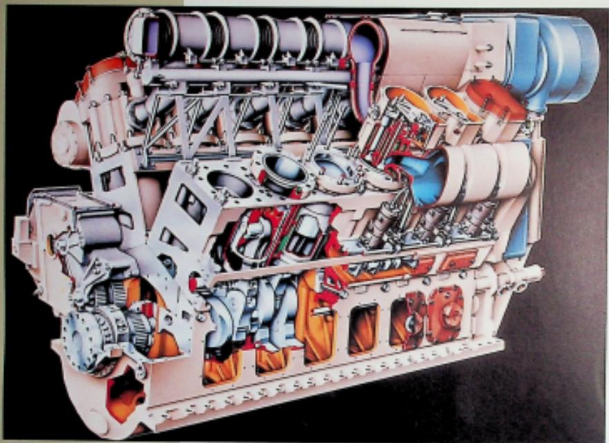
Artist's impression of a medium-speed diesel engine type 12 V 55A.
