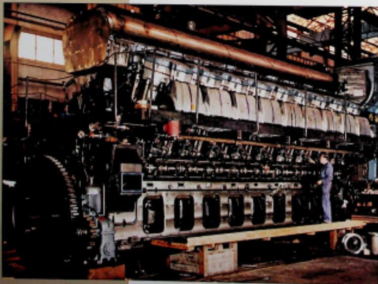
An 18 cyl. four-stroke diesel engine type ACEC-M.A.N. 52/53A during erection.
