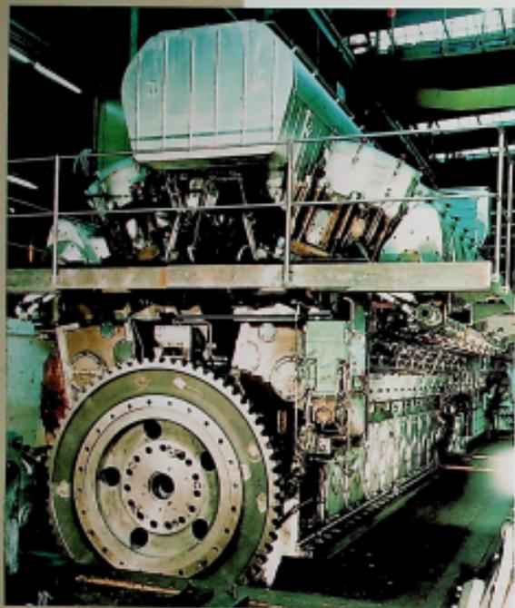
General view of a four-stroke diesel engine type V52/55A (450 rpm - 775 kW/cyl.).
