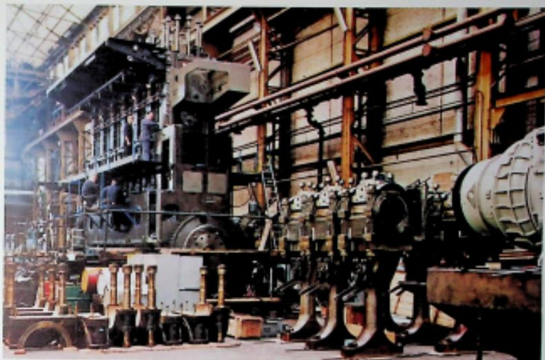
A two-stroke diesel engine type ACEC-M.A.N. K6S2 70/125B (12 400 H.P. - 145 rpm) at test bed. This engine is foreseen for a fruit carrier owned by Ahlers & Partners.
