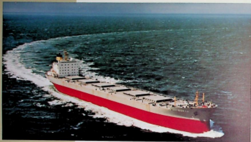
Bulk carrier "MS EEKLO" during sea trials, owned by BOCIMAR and propelled by an ACEC-M.A.N. K6 SZ 90/160A engine (19 200 H.P. - 122 rpm).
