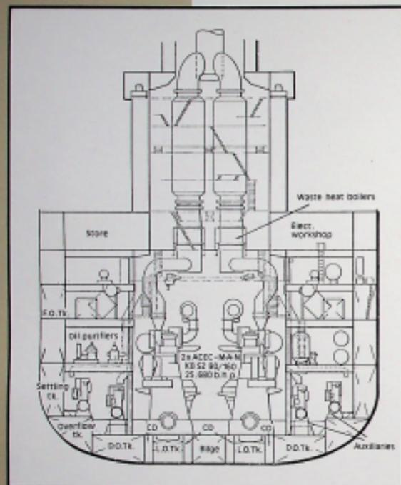
Cross-section of a two-stroke diesel plant.
